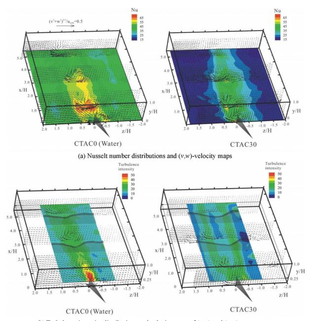
(b) Turbulence intensity distributions and velocity maps of (v,w)-and (u,w)-components
